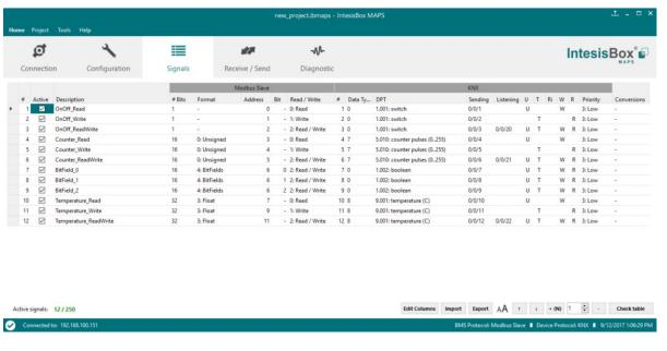
Figure 5.3 IntesisBox MAPS Signals tab
