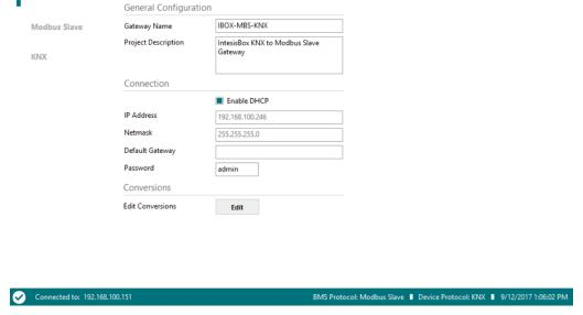
Figure 5.2 IntesisBox MAPS configuration tab
